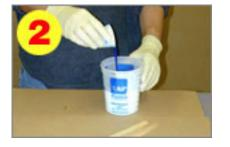
Measure the catalyst and silicone, 10 parts silicone to 1 part catalyst by volume. THOR-OUGHLY mix until there are no streaks. Look at the outside and bottom of the transparent mixing cup. If it is white, more mixing is required. This step cannot be over emphasized! Incomplete mixing will yield inferior results.
