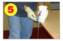
If you do not have a vacuum chamber, there is another method to minimize air in the mold. Cut a 1/2" diameter hold in the side of a cup right near the bottom. Place tape over the hold. Pour the mixed silicone into this cup.
