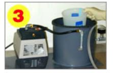
Mixed silicone will be loaded with bubbles (if it is mixed properly). These bubbles can ruin a mold if they are anywhere near the surface of the part. There are two ways to minimize bubbles. The vacuum chamber, pictured here is one method, and step five describes the other.
