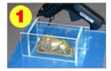
Find or make a container to hold your original part. Container must be leak proof. Construct the container so that the mold walls will be approximately 1/2" thick. Walls thicker than 1/2" make a mold difficult to work with and use more material. Under 1/2" causes the mold to deform when filled with resin.
