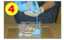
The de-aired silicone is ready to pour into the mold container. Pour slowly into the corner, never over your part. Allow the silicone to slowly flow around the part, thus pushing air out ahead of it rather than trapping air. Deep undercuts may need to be painted with silicone first to minimize air entrapment.
