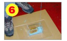
As in #4 above, pour into the corner of the mold and allow the silicone to 'squeegee-gee' air out ahead of it, to minimize trapped bubbles.
