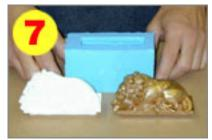
Depending on working temperature, humidity, and catalyst type, your mold will be ready in between 6 and 24 hours. Higher temperature and humidity accelerate the cure. Even though the mold may be usable right away, it continues to cure for a full week. The best castings will be produced after this full cure time, especially if casting in polyester. Quik-Cast is shown in this picture.
